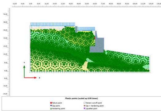
Figure 6.15. Case A - plastic points for undrained behaviour and R_{inter} = 0,5
