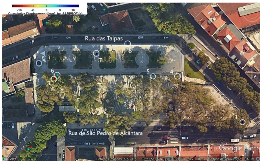
Figure 5.29. InSAR points of displacement measurement in the MSPA (adapted from Roque, 2020)
